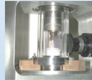
Narrow gap 4-cylinders Couette e=0.1\text{mm}
